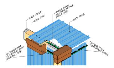
Foam closure are made of rigid polyethylene foam that has very high resistance to ultraviolet rays,can withstand harsh environments and resists some aggressive chemical attacks
